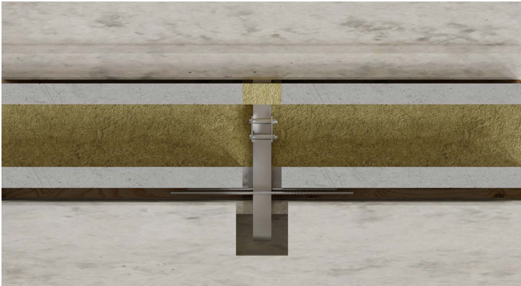
Figure 15. Top view of joint before casting.
