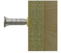
3. When the Ferrule Anchor is fixed with the Nailing Plate to the formwork, it can be filled with concrete. After removing the formwork, the Nailing Plate is visible.
