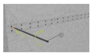
9. Once the bars are assembled in Ferrule Anchors, they are ready for overlapping with the other element reinforcement and pouring the concrete.
