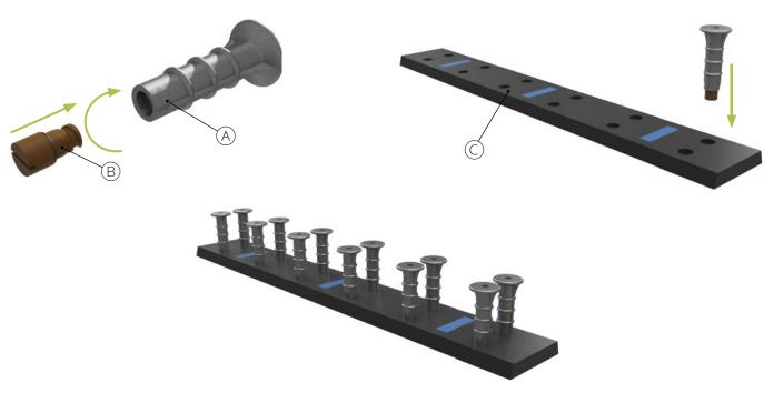
2. After fitting Ferrule Anchors in the right position on the Rebate Former Board, fix ADJUSTA system (Rebate Former Board with Ferrule Anchors) in the required position according to design by attaching it with nails onto the wooden formwork or connecting it to the existing reinforcement of the concrete element with wires.
