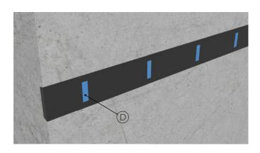
6. Remove the Rebate Former Board by using the Board Release Key (see Annex B - Accessories).
