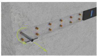
8. Easy fitting of Threaded Bars © to Ferrule Anchors by screwing in. Threaded Bars are fully tightened when the colored part of Threaded Bar is completely hidden in the Ferrule Anchor.
