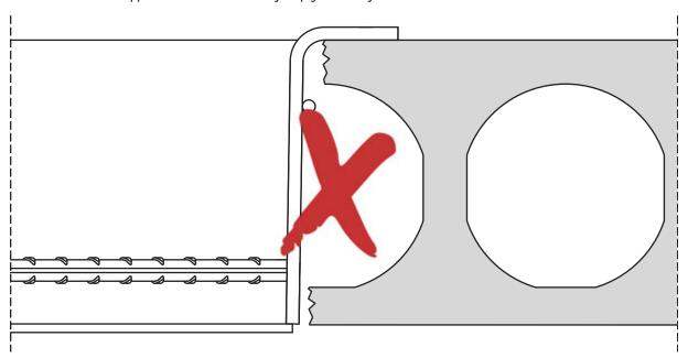
Two hollows must be connected, reinforced, casted and designed to support PETRA when there is a need to support PETRA on the area of hollows.
