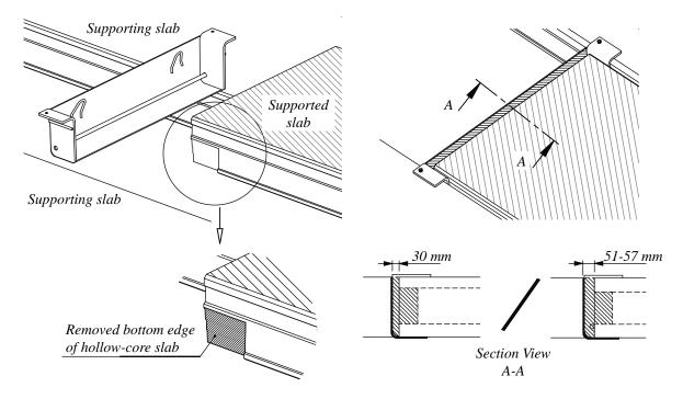
The bottom edge of the supported slab should be removed so that the slab bears directly on the front plate. The top flange of the side plates of the PETRA contains  $\emptyset$ 12 mm holes for fastening PETRA to supporting hollow-core slabs using expander bolts.
