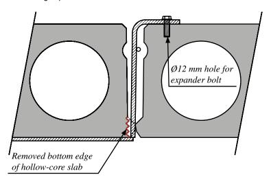
The gap between PETRA and the hollow-core slab should be fully cast when concreting the floor. The concrete should be hardened before applying loads to the floor. Lifting loops welded on the front plate are used in the manufacturing and shipping process. They can be removed before PETRA is installed on-site.
