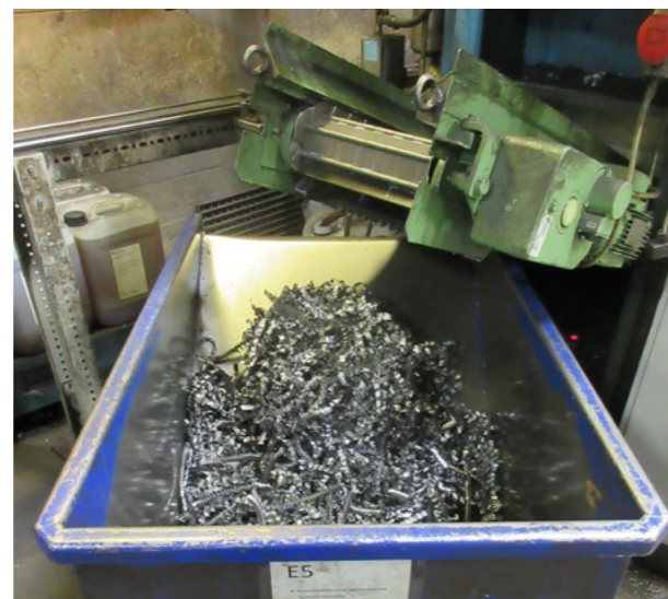
Photo steel scraps from drilling, waiting to be send to a steel mill to become reused circular.
