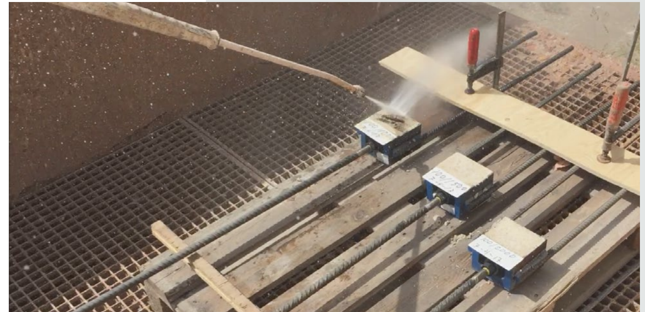
Photos showing the tests for Peikko SUMO® Wall Shoes. These connections were cast with different strengths of lime mortar.
