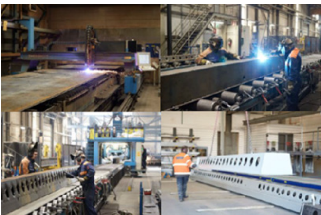
Figure 5. Manufacturing processes of DELTABEAM®.
