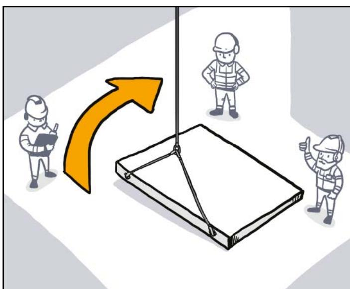
COMPATIBLE ANCHORS for tilting up a wall
