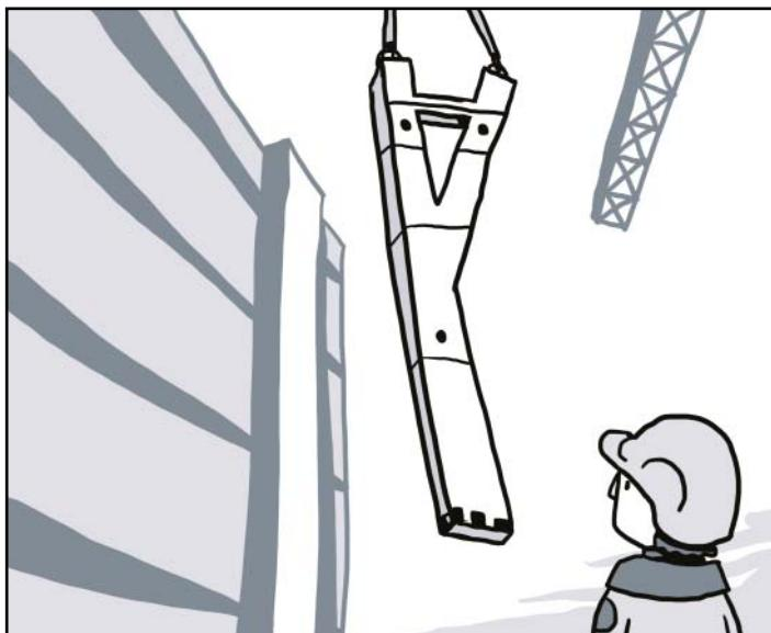
COMPATIBLE ANCHORS for lifting a column
