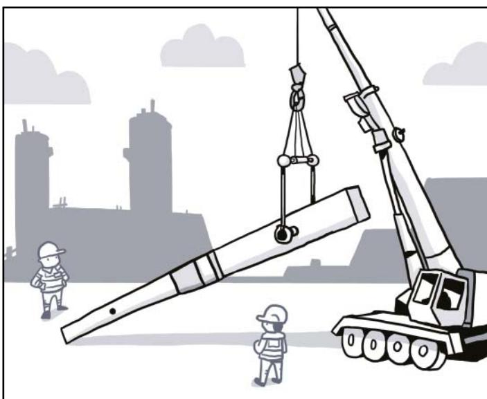
COMPATIBLE ANCHORS for tilting up a column
