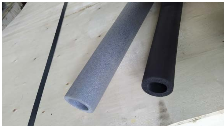
Figure 7. Closed-cell foam tube for VOLT BOLT®.
