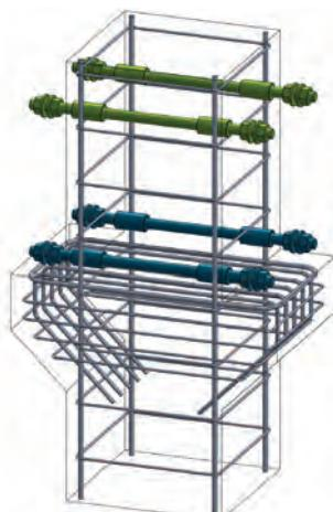
COPRA Anchoring Couplers in a double-sided beam-to-column connection
