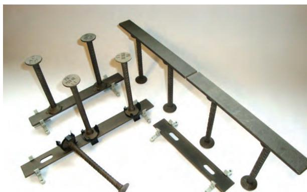
Double headed studs, assembled by a flat profile as spacing bar. Available as 2 and 3 studs elements or long 2-10 studs on flat profile. Flat profile has no load bearing function, it only guarantees the correct spacing and positioning of the studs during installation. Available in diameters 10, 12, 14, 16, 20, 25, 28 and 32 mm.
