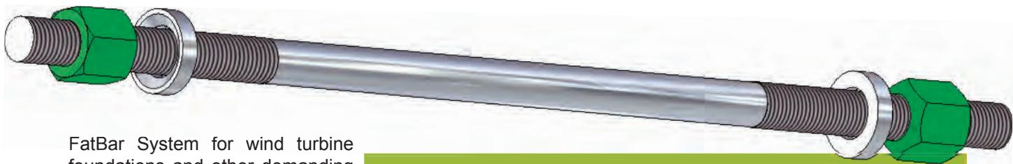
FatBar System for wind turbine foundations and other demanding engineering applications sustains fatigue loads by ETAG 13 test with ease. The FatBars are post tensioned against high dynamic stress and thus protect the foundations from cracking even in harsh conditions. Optionally, FatBar bolts can also be ecologically corrosion protected by ECO Galvanizing to increase the life time of the foundations.
