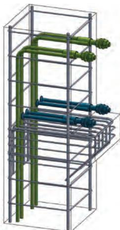
COPRA Anchoring couplers in a single-sided beam-to-column connection
