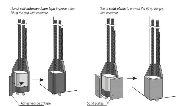
Ensure of thicker concrete cover by self-adhesive foam tape or solid plates
