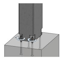
After the nuts are tightened, the crane can be released
