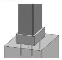
In column to foundation connections wider grouting can be provided to ensure higher concrete cover if it is required. It is recommended to increase the cover in aggressive environment.
