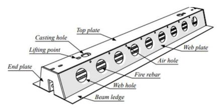
DELTABEAM® consists of steel plates welded together into a delta kind of shape. It is a steel structural element which can be combined with all general concrete slabs, steel decking and wooden slabs. It is integrated into the floor and filled with concrete on-site. The infill concrete and
