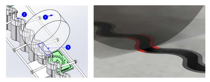
Figure 1. Example: Ø250 × 100 wheel ① is crossing WAWEJOINT®, joint opening 20 mm ②, pressure area of wheel 30 × 100 mm<sup>2</sup> ③. When crossing the WAWEJOINT®, the wheel carries on/from both sides of slab at the same time.
