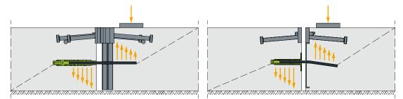
Figure 3. WAWEJOINT® and TERAJOINT® dowels have similar Load Transfer.
