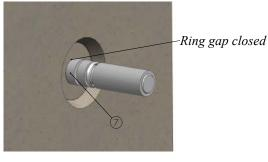
3. Align the thread of coupler Part B  $\bigcirc$  of the MODIX<sup>®</sup> PM  $\bigcirc$ .
