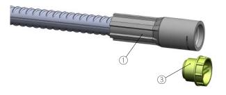
3. MODIX<sup>®</sup> Part A ① is screwed to the nailing plate N or magnetic plate M. It is recommended that lubrication be applied to the thread of MODIX<sup>®</sup> Part A ① to avoid pollution from fresh concrete and also for better handling when removing the thread protector from MODIX<sup>®</sup>.
