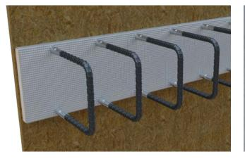
Remove the ARBOX<sup>®</sup> steel cover by cutting the tapes that secure it, then place the claw of a hammer at one end and pull it away. Remove bolts inside of the steel box by wrench.
