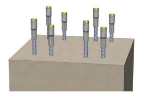
1. If MODIX<sup>®</sup> must be installed at the casting level (e.g., due to construction requirements), it is recommended to use lubrication around the thread protector to avoid pollution from the fresh concrete and also for better handling when removing the thread protector from MODIX<sup>®</sup>.
