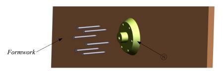
2. Directly before installing MODIX<sup>®</sup> Part A 1, remove the thread protector 3 from the coupler.
