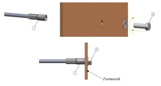
3. After removing the formwork, screw back the thread protector ③. It must be removed directly before assembling the counterpart.
