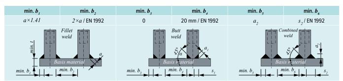
Standard weld, no preparation neededButt + Combined weld are special cases, welding seam preparation to be appliedmin.  $b_2$ , min.  $b_4$ , min.  $b_6$  = consider EN 1992 + NA chapter 8.2, to check maximum of  $\{k_1 \times \emptyset; k_2 + dg; 20 \text{ mm}\}$
