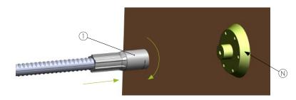
4. When MODIX<sup>®</sup> Part A ① is fixed with nails or a magnetic plate, the formwork can be filled with concrete. After removing the formwork, the nailing plate 🕅 or magnetic plate 🕅 is visible. After the fixation plate is removed, MODIX<sup>®</sup> Part A is ready for assembly with the counterpart.
