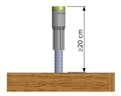
The threads of the MODIX<sup>®</sup> couplers must be protected by thread protectors during casting. Remove the thread protectors only directly before installing the counterpart couplers.
