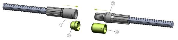
3. Coupler Part B ② is screwed onto coupler Part A ①. Carefully turn Part B ② on the first pitches into Coupler Part A ①. Never use force to connect coupler Part A ① and coupler Part B ③. Correct use enables a screw connection to be made by hand.
