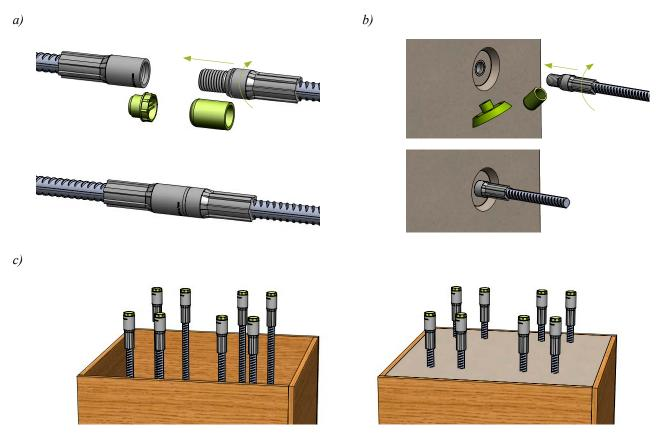
Figure 1. a) MODIX<sup>®</sup> connected inside concrete elements MODIX<sup>®</sup> connected on the surface of the element, b) attached to formwork, c) protruding bar solution.
