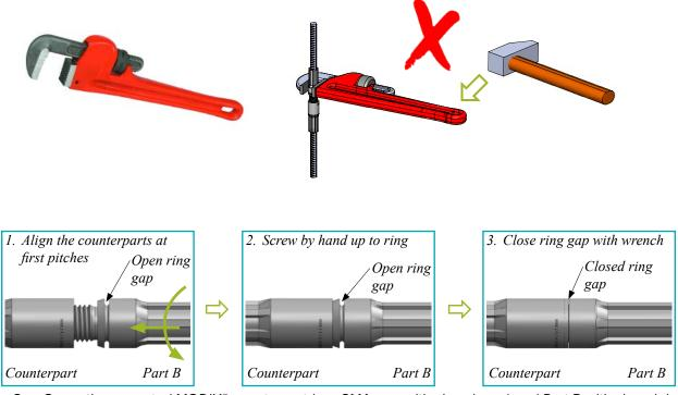
Figure 2. Correctly connected MODIX<sup>®</sup> counterpart (e.g. SMA or positioning sleeve) and Part B with closed ring gap.
