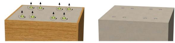
2. If MODIX<sup>®</sup> is installed at the casting level and used in an environment where there is risk of damage to the plastic thread protector (e.g. in an area where there is the movement of heavy vehicles) after the concrete has hardened, it can be substituted with an M-thread bolt. It is recommended that lubrication is used around the bolt to facilitate the removal of the bolt.
