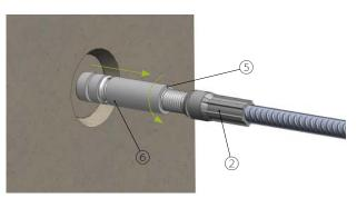
4. Turn the positioning sleeve (6) until the ring gap is closed. The second counter nut (7) is then tightened against the positioning sleeve until the ring gap is closed.
