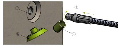
2. Coupler Part B ② is screwed onto coupler Part A ① (already cast in the concrete element). It is tightened using a wrench until the ring gap is completely closed.
