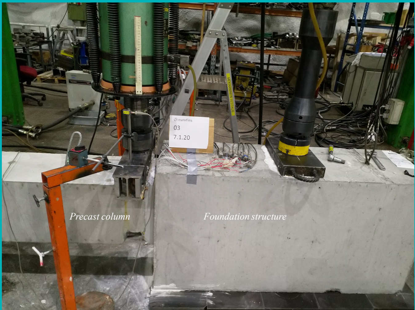
Figure 6. Test setup of one of the shear tests.
