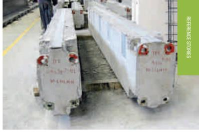
Shoes were used, depending on the bending moments existing in each joint and always trying to standardize the solution as much as possible.
