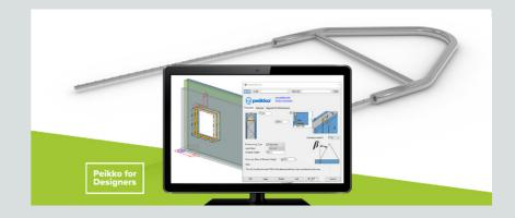
only place one insert at a time. The WILJA® Lifting Insert type can either be selected automatically, or manually by the user. During automatic selection, the user must define the inclination angle, dynamic factor, and load share (weight share of the element) for one Lifting Insert as a percentage, as these will affect the background calculations. The choice of inclination angle will also ensure that the user receives additional diagonal reinforcement in the wall, as needed.
