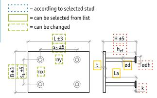
Modified WELDA<sup>®</sup> Fastening Plates must be named such that they cannot be confused with standard WELDA<sup>®</sup> Fastening Plates. Manufacturing drawings are required for production. The drawings must show the dimensions of the plate, the sizes and positions of the anchors, and the materials. Contact Peikko's sales team for more information about modifying WELDA<sup>®</sup> Fastening Plates.
