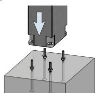
The upper nuts and washers are screwed onto the bolts
