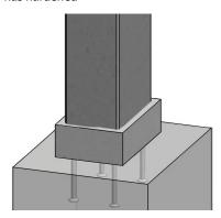
In column-to-foundation connections, wider grouting can be provided to ensure higher concrete cover if it is required. It is recommended that the cover be increased in aggressive environments.
