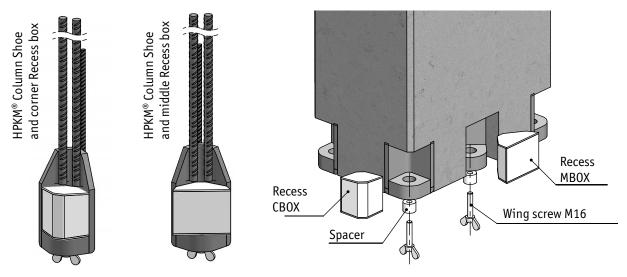
To ensure higher values of concrete cover thicknesses of main anchor bars in accordance with section 1.2.3 of the technical manual, follow these instructions for increased values  $\Delta_c$  of concrete cover:
