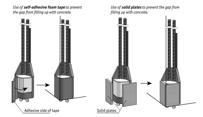
Ensure thicker concrete cover using self-adhesive foam tape or solid plates.
