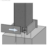
Finalized connection after grouting has hardened
