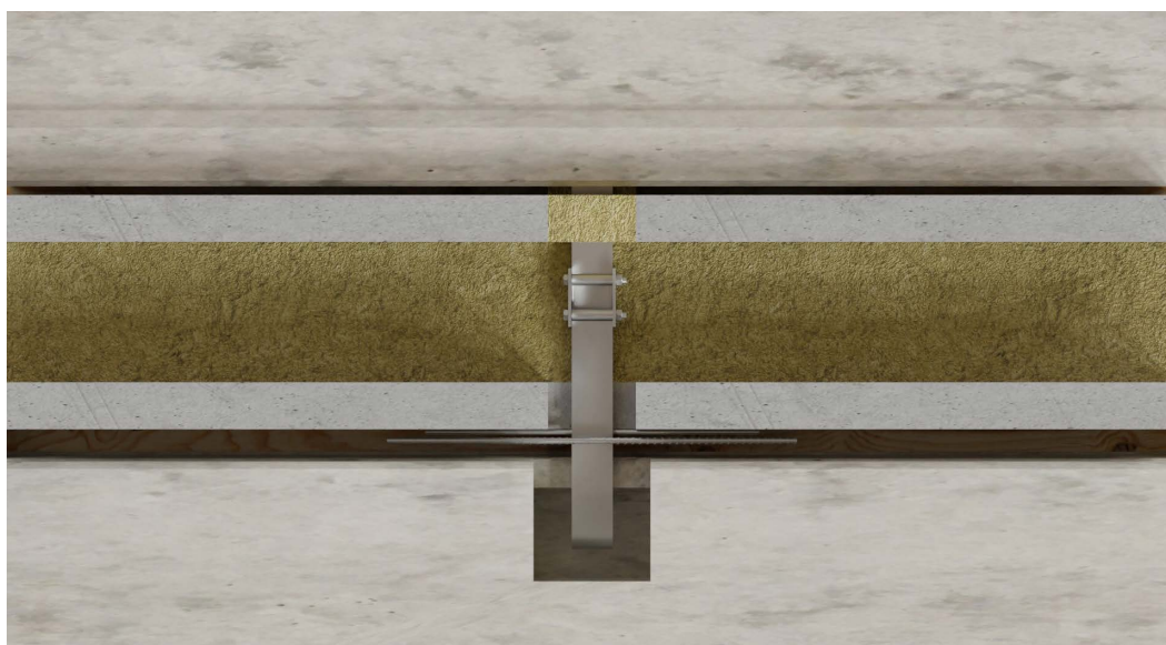
Figure 15. Top view of joint before casting.
