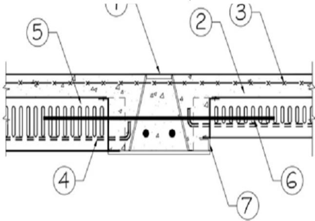
1. **Structural Steel Member\*** — Composite beam system. Min. bearing 2 in.
