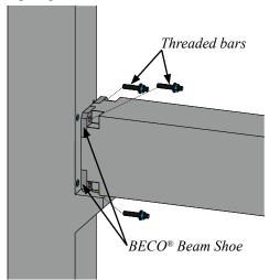
The connection is finalized after the grout has hardened.
