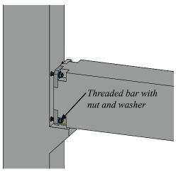
Insert the threaded bars with washers and nuts through the base plates into the coupler parts of the anchoring couplers.
