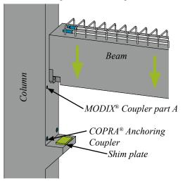
Fill the connection with grout and screw on the MODIX® Rebar Couplers.
