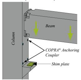
Screw the nuts, washers and threaded bars on and tighten them.
