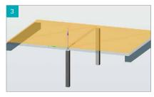
3. Define the beam length and choose slab types and spans
