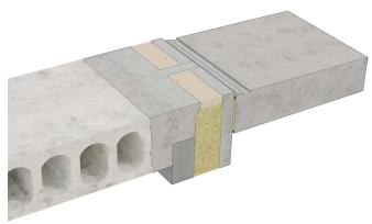
4. Pour the concrete into the formwork and fill the void between floor slab and wall panel. After the concrete reaches the required resistance, remove the formwork. SLADEX® carries full load from the precast slab into the base structure.
