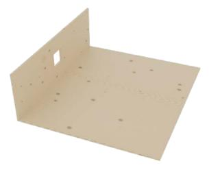
1. Prepare formwork and cut the opening for the RHS tube profile.
