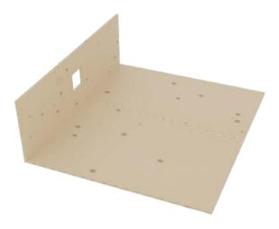
1. Prepare the formwork and cut out the opening for the RHS tube.
