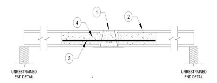
1. Structural Steel Member \* — Composite beam system. Min depth 8 in. Min bearing 4-1/2 in.
