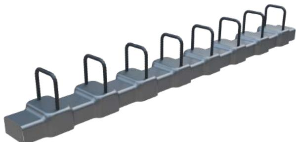
Model with two rows of anchor bars where the straight part of the reinforcement is bent inside the box
