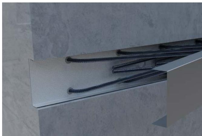
Straighten the bars using an appropriate re-bending tool (e.g. pipe with internal diameter not greater than  $2 \times$  nominal bar diameter). **Bars must only be straightened once.**
